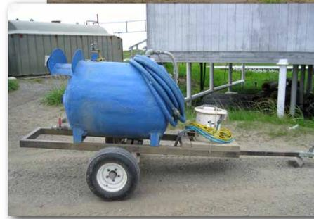
FIGURE 4 (above). Flush tank and haul sewage tank, commonly known as "a dog house."
