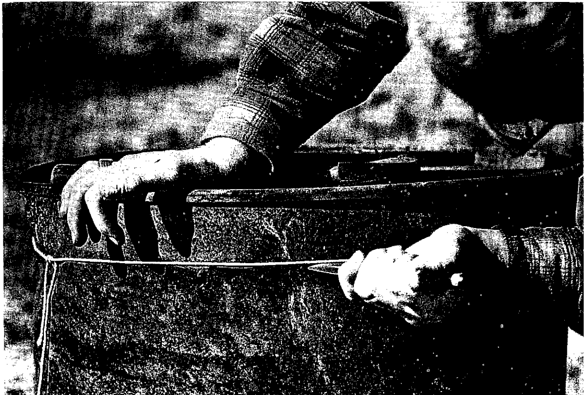
2. MARK A LINE AROUND THE BARREL
