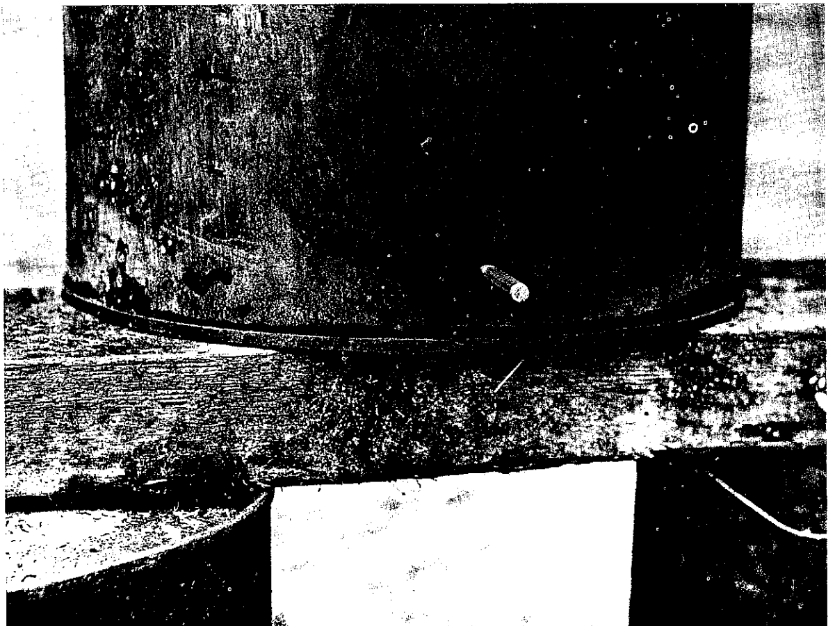
11. HAMMER PUNCH THROUGH TO MAKE HOLE
