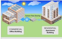
District-scale energy modeling will allow buildings with complementary loads to be matched together to utilize common mechanical equipment most efficiently.
