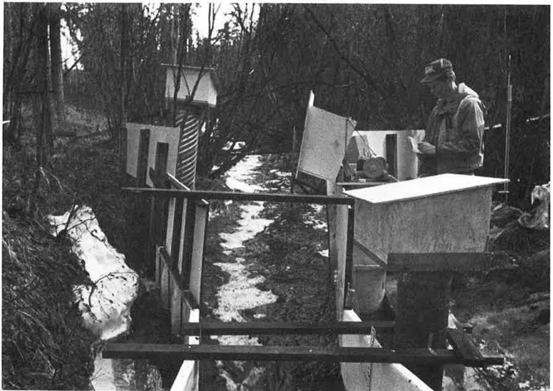
USDA researchers monitor spring runoff at Spinach Creek watershed near Fairbanks, Alaska, to develop ways of predicting spring runoff patterns in relation to topography, climate, and land use.
