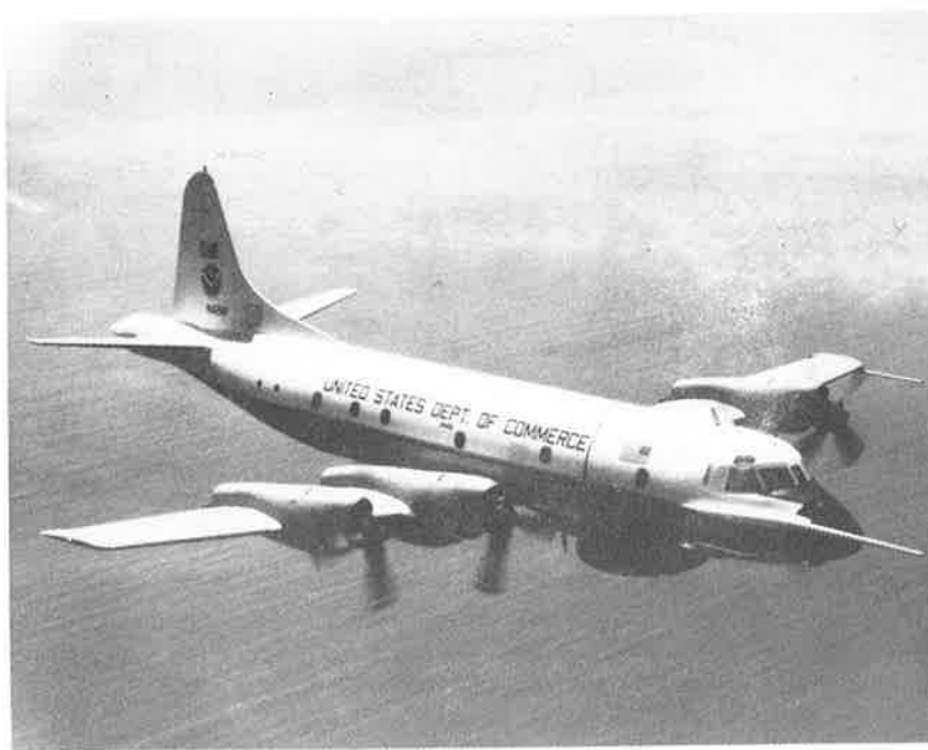
The National Oceanic and Atmospheric Administration WP-3D Orion research aircraft used in the Arctic Gas and Aerosol Sampling Program. This aircraft is capable of 10- to 12-hour research missions with a range of more than 3000 nautical miles.
