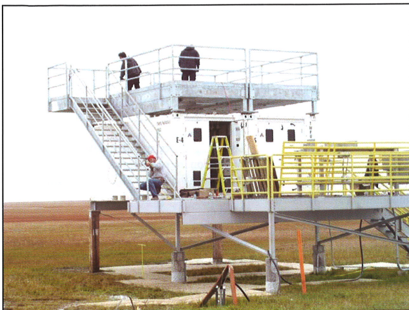
Additional instrument shelters and topside deck for "visiting" upward-looking instrumentation installed at the Barrow, North Slope of Alaska ARM Climate Research Facility during FY 2005.
