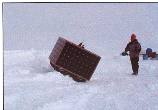
Cool Robot climbing a 0.3-m-high, steep-faced snow berm at Summit Camp, Greenland.
