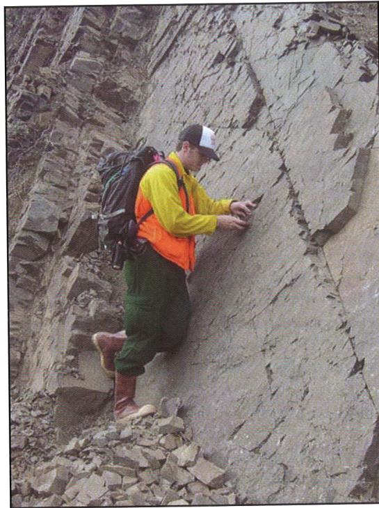
GeoCorps intern measuring the strike and dip of exposed bedrock at Canyon Creek.
