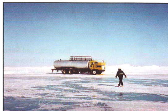
Water spray truck drawing water from a local North Slope lake. Trucks like this are used to create the ice roads.
