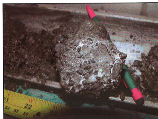
Sample of core material, recovered from the Mallik Research Consortium drilling effort, showing the presence of gas hydrate (white).
