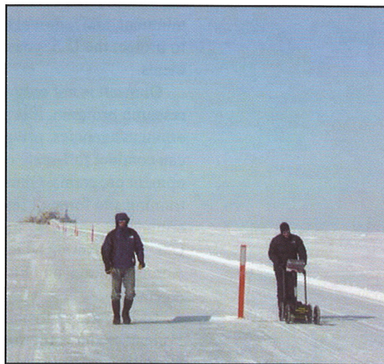
Radar team at Prudhoe Bay in April 2005 during cold weather reliability trials and thick ice (up to 6.5 feet) profiling without oil.
