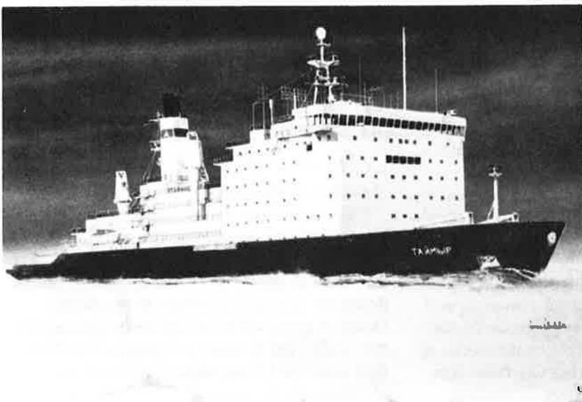
Artist's conception of the Taymyr, a Soviet shallow-draft, nuclear polar ice-breaker under construction in Helsinki by the ship-builder Wartsila.
