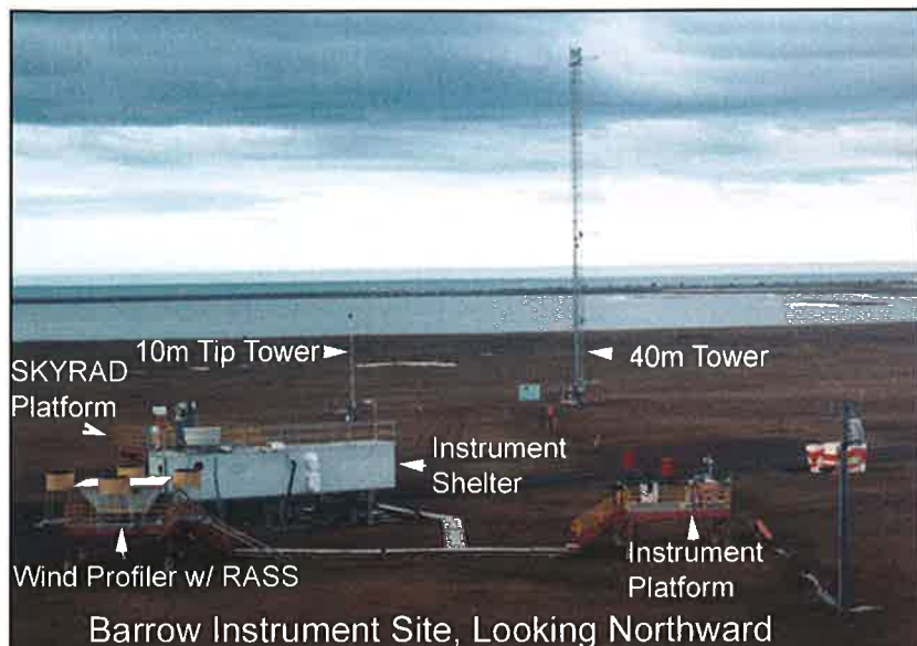
Low-level aerial view of the ARM Climate Research Facility (ACRF) Barrow site. See http://www.arm.gov for a description of the instrumentation.
