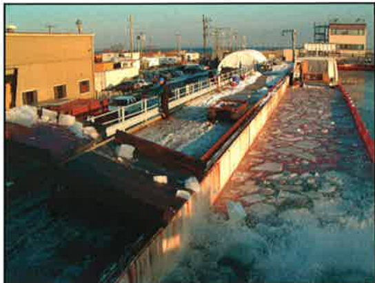
Preparing Ohmsett for mechanical oil-in-ice experiments.
