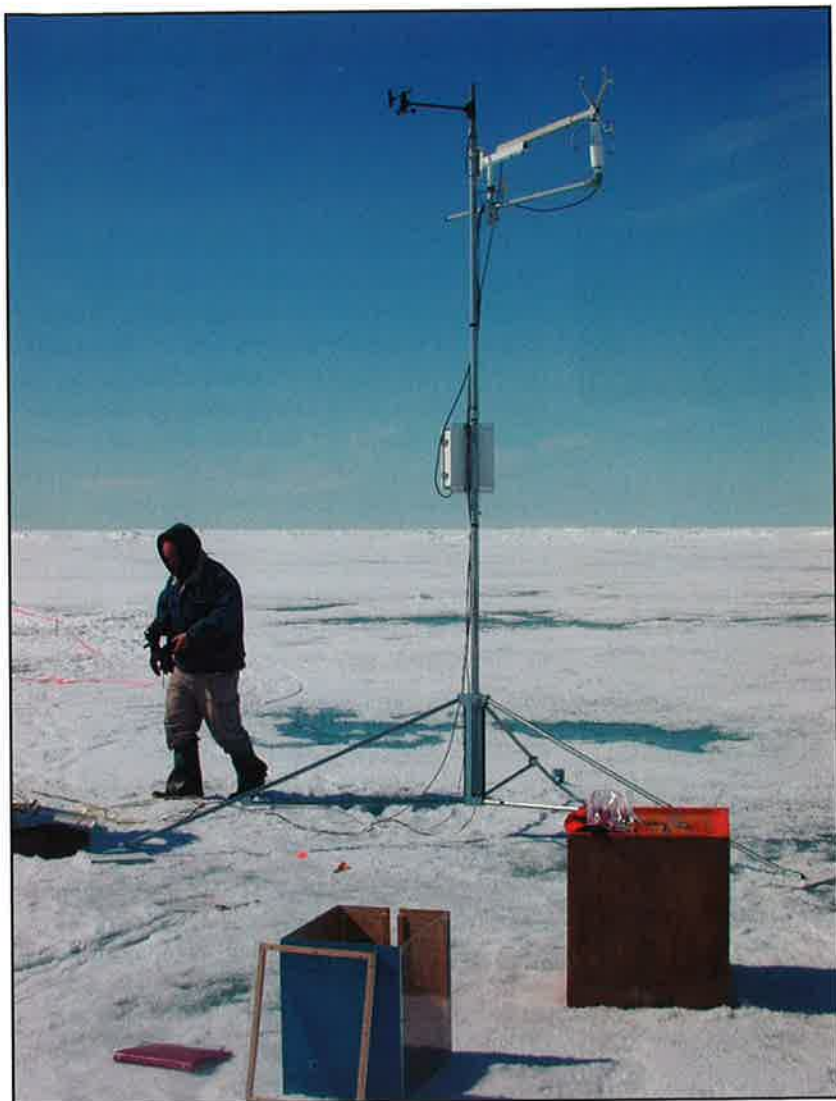
Eddy-correlation measurements of the carbon dioxide flux and other turbulence quantities on the fast ice near Barrow, Alaska, June 2002.
