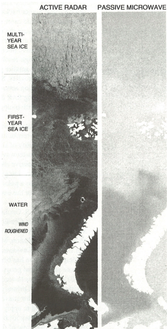
Simultaneously acquired real-aperture side-looking radar and passive microwave images of the Barents Sea region collected by the Russian Okean-07 satellite, 2 January 1997, 16:40 UT.
