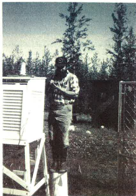
Forest Service technician changing a pollen slide at an LTER weather station on the floodplain of the Tanana River in the Bonanza Creek Experimental Forest.
