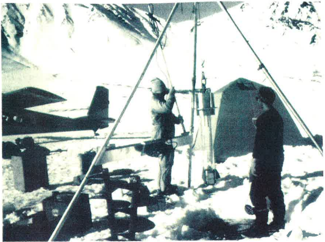
Collecting sediment cores from the surface of the ice at Cascade Lake, North Slope Borough, Alaska, in the spring of 1994.
