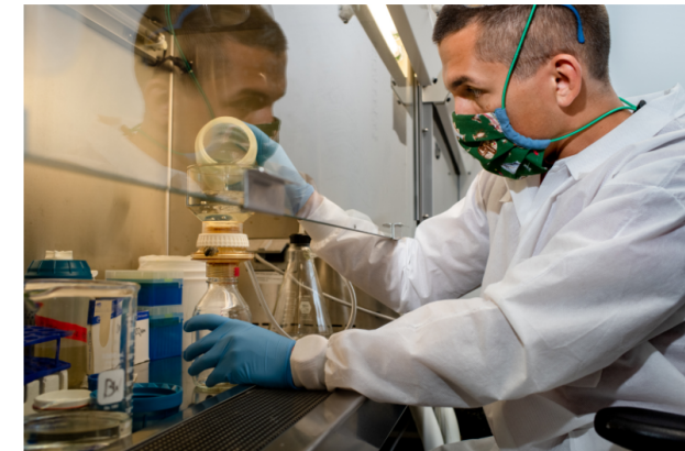
Arden Nemudryi, a postdoctoral researcher at Montana State University, uses a bottle top filter to separate SARS-CoV-2 virus RNA from a waste water sample. Mike Greener/High Country News
